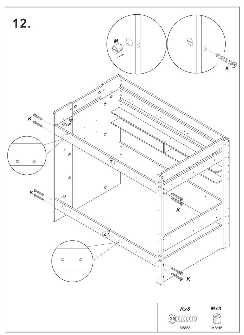
**Note:** on panel 7, the holes are not punched through so that the ladder side can be switched as needed, please use drill bit or the provided wood screw (A) to drill through to widen the holes.
